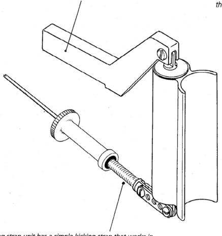
This version of the gooseneck/kicking strap unit has a simple kicking strap that works in tension only.
